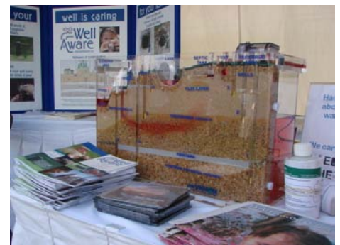
The red is a containment moving through the native soils – an excellent visual tool to see what goes on under our feet.
